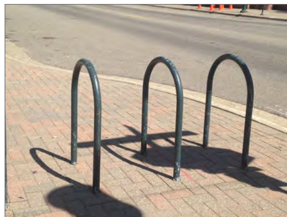
Recommended Inverted-U style bicycle racks in Downtown Robbinsdale.
