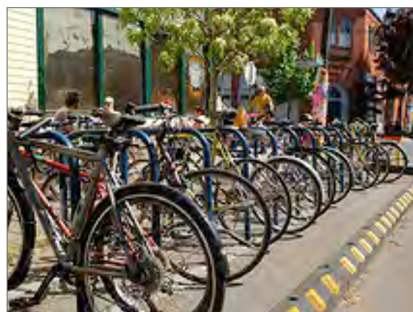
On-street bicycle corrals may be used in lieu of vehicle parking spaces where bicycle traffic is high. Corrals can park 10+ bicycles. Installing corrals at corners provides curb extension benefits for pedestrians as well. Image courtesy of J. Maus and bikeportland.org.
