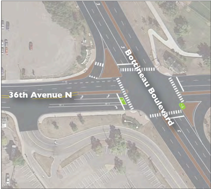
Proposed: Continue bicycle lanes along 36th Avenue N to Bottineau Boulevard, reduce excess turn lanes, extend medians to provide pedestrian crossing refuges, and modify right-turn slip lane design to improve conditions for pedestrians and bicyclists.
