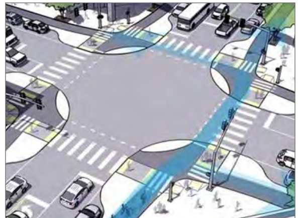
A rendering of protected intersection for bicyclists. Elements such as advance vehicle stop bars, corner refuge islands, setback bike crossings, and bicycle-specific signals are included in this concept. Image courtesy of protectedintersection.com
