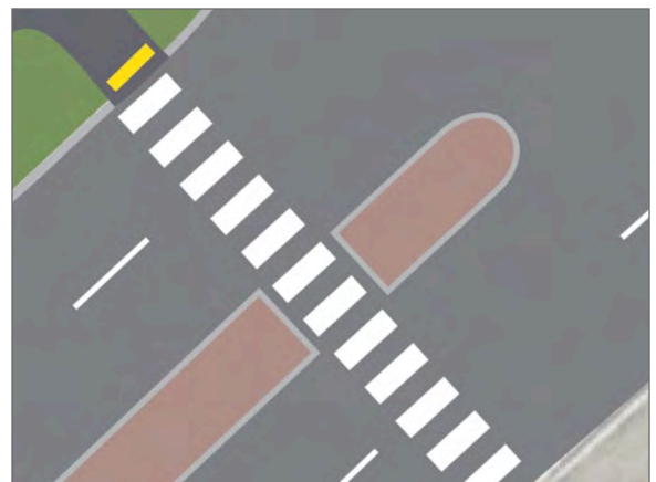
A “bull-nose” refuge island is created by extending the median beyond the crosswalk.
