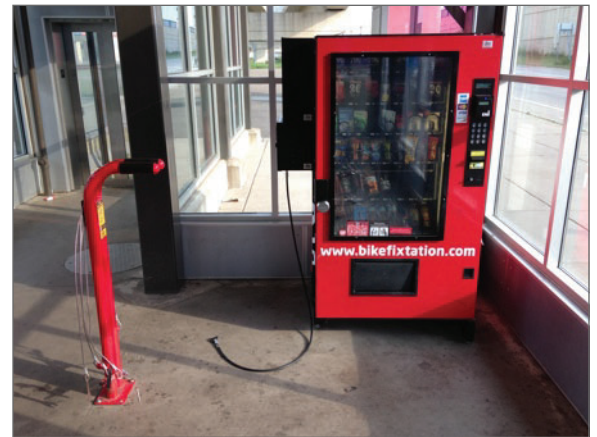
This fix-it station provides basic bicycle repair tools and parts with a vending machine and permanent repair stand.
