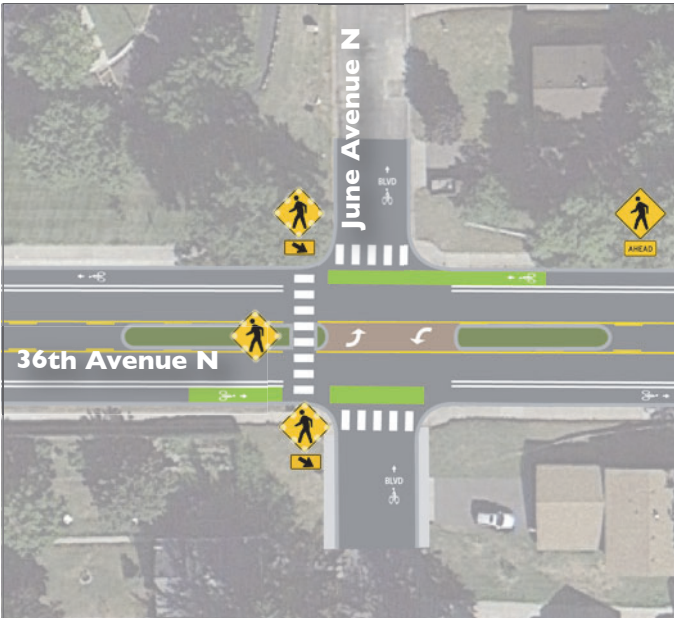
Proposed: High visibility crosswalks, traffic calming pedestrian refuge medians, and pedestrian crossing signage improve visibility, safety, and comfort. Note that this concept rendering also assumes modifications to 36th Avenue North proposed in the route recommendations of the next section.
