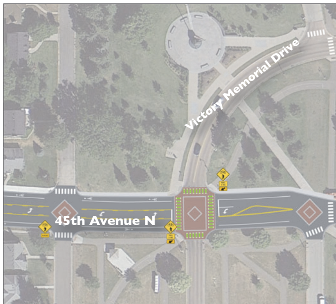
Proposed: Sidewalk improvements, on-street bicycle facilities, and plaza-inspired intersections improve conditions for pedestrians and bicyclists.
