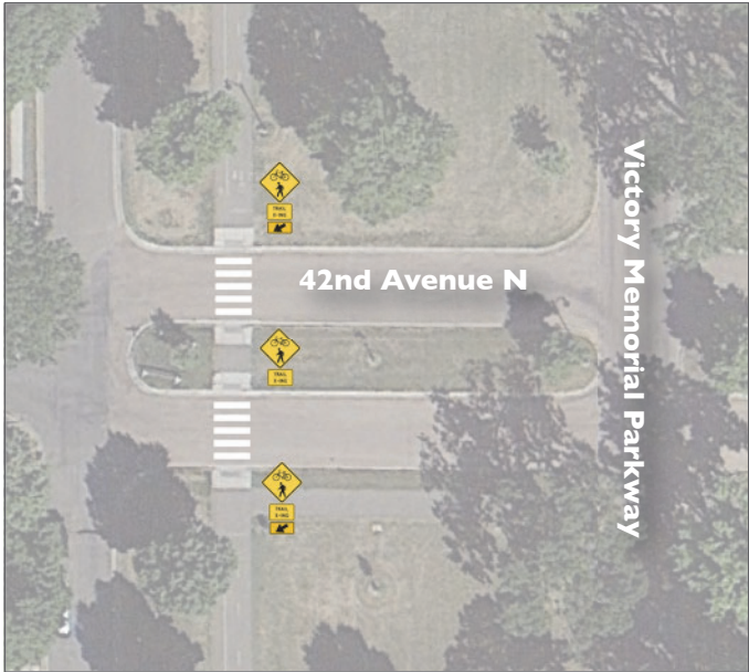
Proposed: High visibility painted crosswalks and trail crossing assemblies improve visibility of trail users crossing the street.
