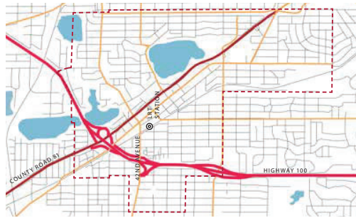
Fig. 11 LOCAL STREET PATTERNS The city is characterized by a grid of local streets that is interrupted and distorted by Highway 100, County Road 81, a freight rail corridor, and natural features, such as lakes. All of the disruptive elements have limited crossing points, funneling traffic onto a few crucial arterial streets.
