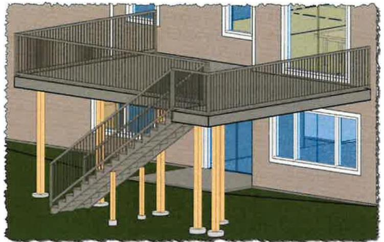
pressure (MRC Table R401.4.1). The minimum depths of footings must be either 5'-0" (Zone 1) or 3'-6" (Zone 2). Refer to Minnesota Rules 1303.1600 for the counties included in each zone.
